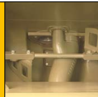
Tolva con válvula "S" con disco y placa de desgaste Hopper with "S" valve with disc and wear plate
