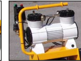
Compresor monofásico de 220 l/min. Single-phase compressor 220 l/min. output.
